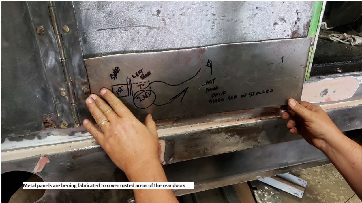
Metal panels are being fabricated to cover rusted areas of the rear doors
