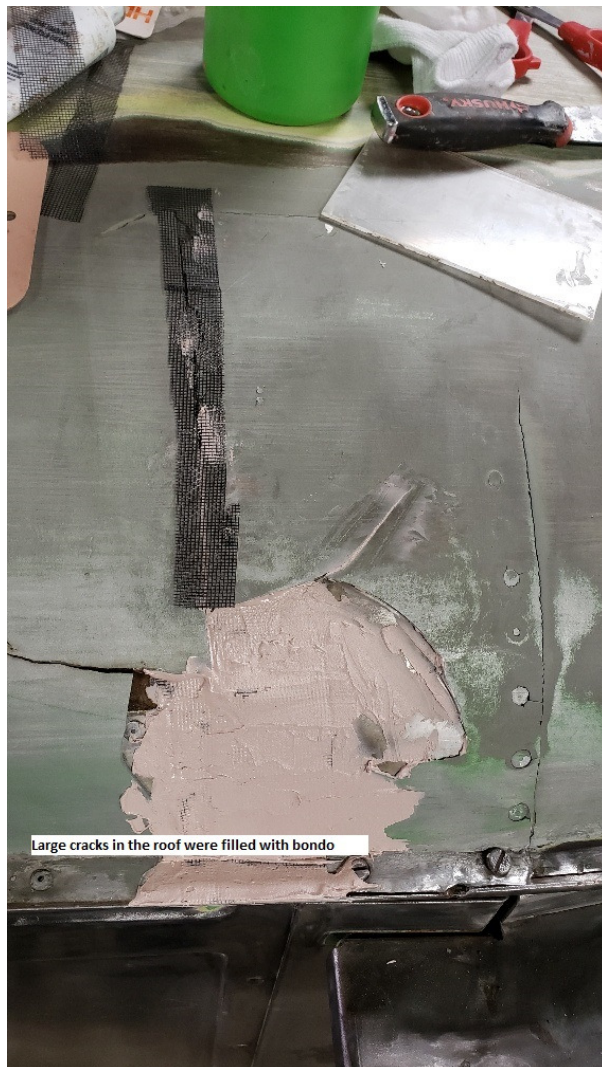
Large cracks in the roof were filled with bondo
