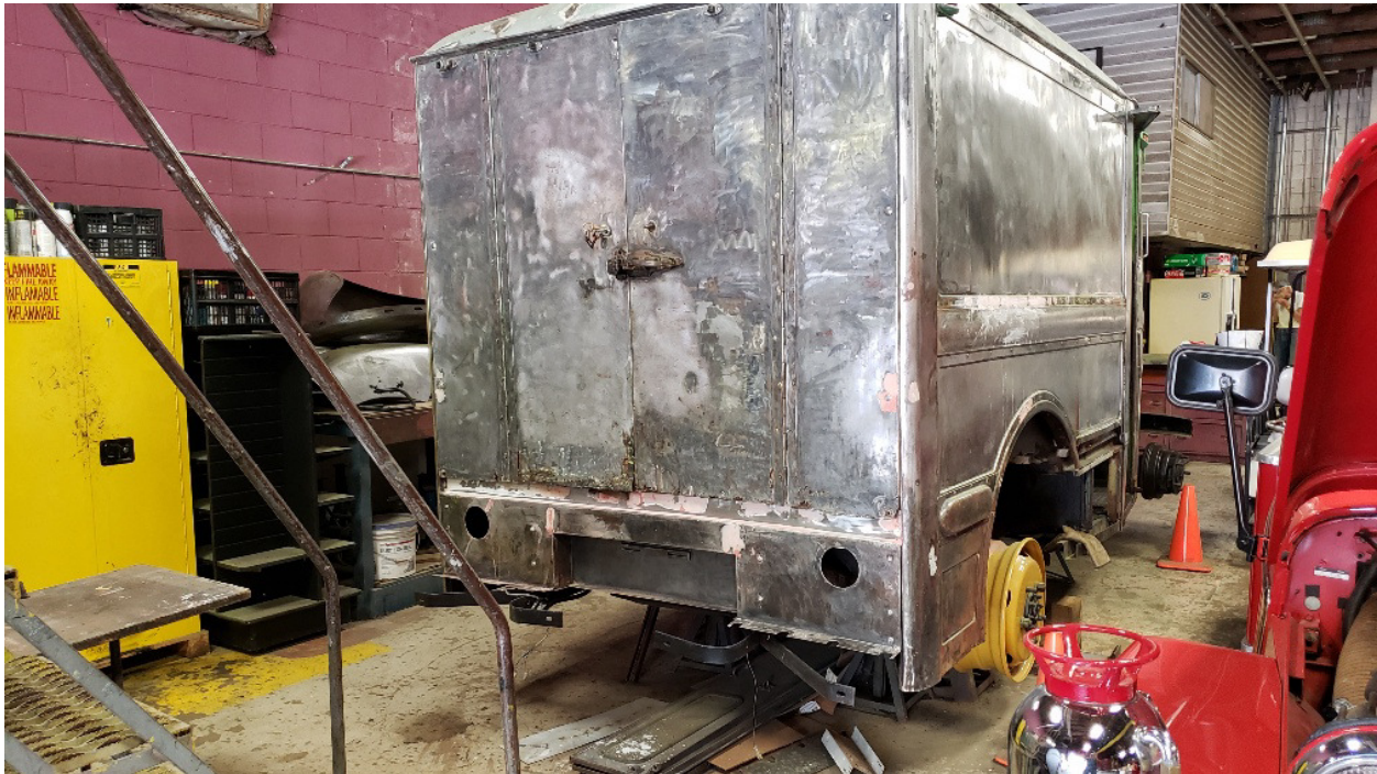
Bondo repair of The rear filler panel between the floor and tail light/license plate panel was completed
