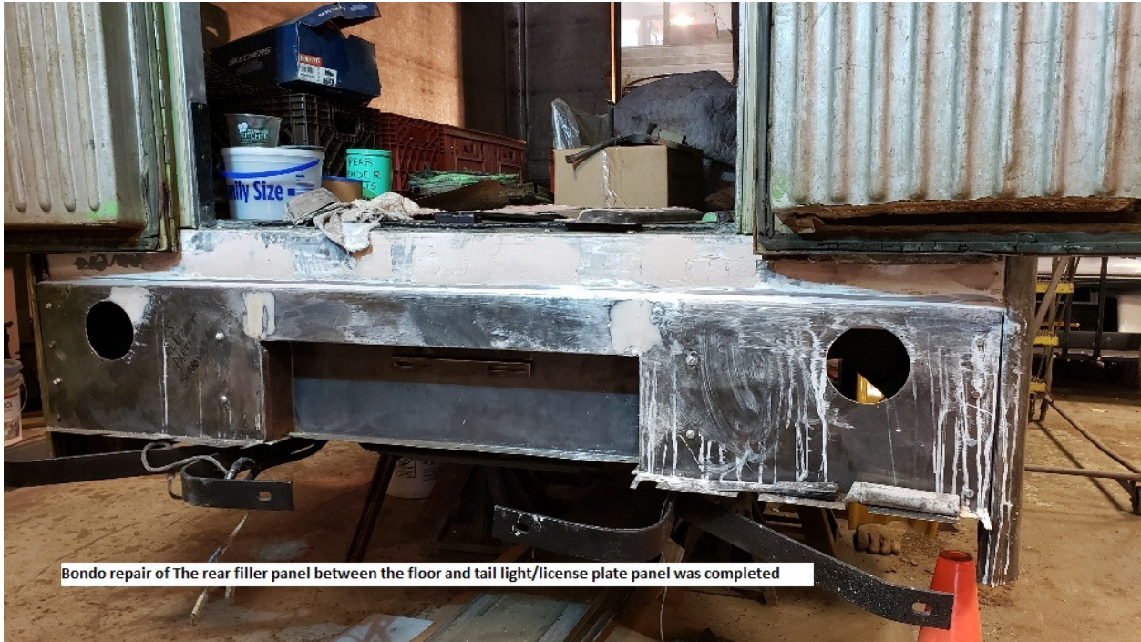
Bondo repair of The rear filler panel between the floor and tail light/license plate panel was completed
